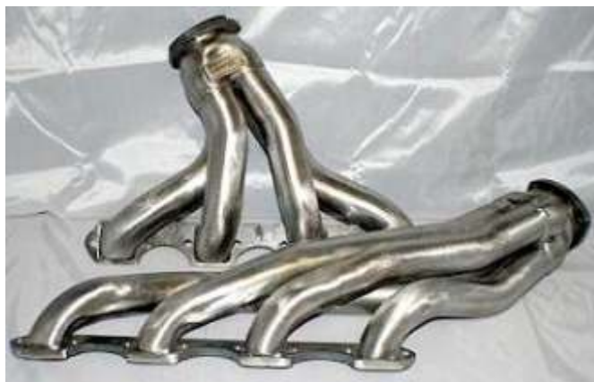
EX52 - 1968 - 1979 Deville Headers, plain. Slight chassis modification required for 1977-79 Deville's.
